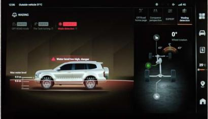
**Wading Depth Detection** Water depth detection system
